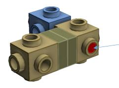
Make sure that the end of the pin stays aligned with the top of the stud (flushed)
